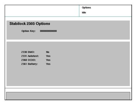
If you purchase a new software option as an upgrade, you will receive an option key. This key is a sequence of alphanumericals that allow you to install the option quickly on your workbench, without the need to ship it to a Willtek service center.
