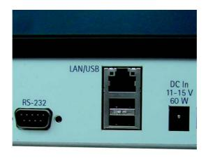
In addition to operating the 2303 Stabilock through its front panel elements, it can also be controlled remotely from a PC through the serial (RS-232) interface or the LAN (local area network).
