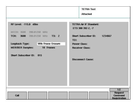
6 Push **Call** to set up a voice channel and activate the loop. The Call Active menu appears. You can now switch between different views and observe the measurement results.
