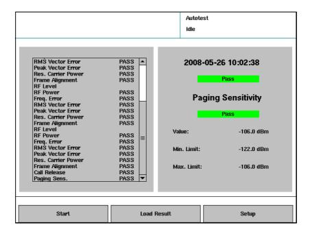
3 In the progress section, highlight a short-form result or test step. Details regarding the short-form result or test step are shown in the details section.
