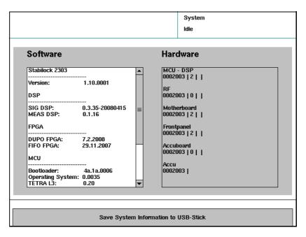
Insert a USB flash drive into a free USB slot and push **Save System Information to USB Stick**.
