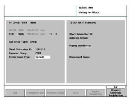
5 Switch on the MS and wait until the 2303 displays Attached in the upper right corner.
