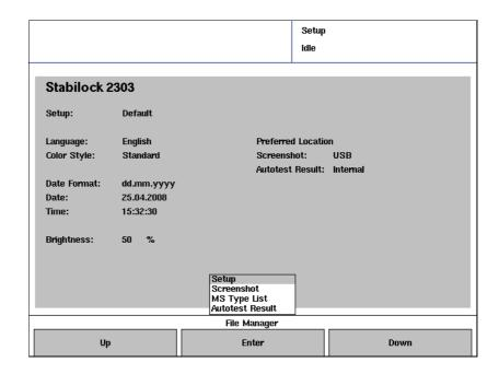
2 Select the desired file type and press ENTER. The corresponding File Manager menu appears, on the left-hand side displaying the available files that are stored on the Stabilock and with the files in the corresponding folder of the USB or NFS drive on the right-hand side.
