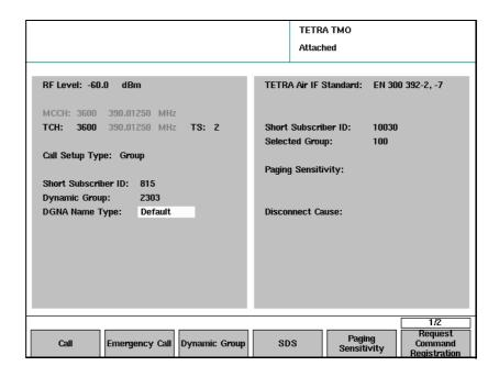
6 Set up the call parameters as explained in "Setting up the call parameters" on page 16. In particular, enter the call setup type and Short Subscriber ID; the dynamic group number is not required in an individual call.
