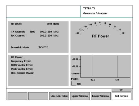
4 Select a signal type in the Downlink Mode field: TCH 7.2 (the 2303 transmits four time slots per frame, one containing a typical TCH/7.2 signal, the other slots filled with dummy bursts) SCH/F (the 2303 transmits four time slots per frame, one containing a typical control channel; this signal is useful for MER measurements) **BSCH + SCH/HD** (the 2303 transmits four time slots per frame, one containing a BSCH + SCH/HD signal with a PRBS, the other slots filled with dummy bursts)
