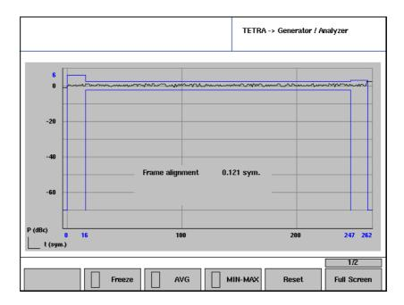
When you are finished with the full-screen burst profile display, return to the Generator / Analyzer menu by pushing the **ESC** button.
