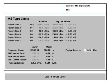
You may want to push the **Load RF Power Limits** softkey to select the power class of the TETRA radio to be tested.
