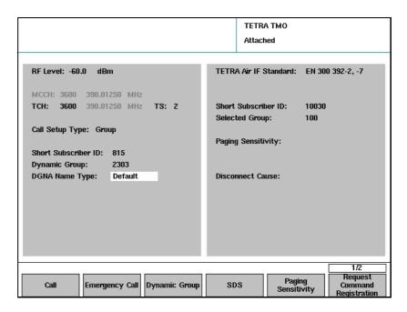
6 Set up the call parameters as explained in "Setting up the call parameters" on page 16. In particular, enter the call setup type and the dynamic group number; the Short Subscriber ID is not required in an incoming group call.
