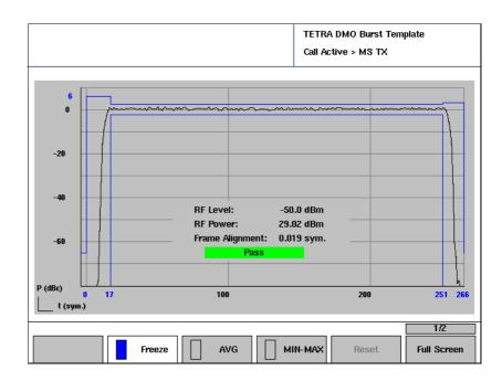
Chapter 4 Testing the TETRA Radio in Direct Mode Performing transmitter measurements
