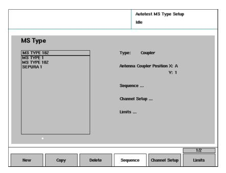
2 From the list on the left-hand side, select an entry that corresponds to the type of mobile station to be tested.
