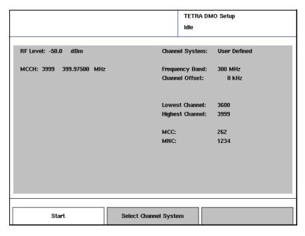
3 Push the **Select Channel System** softkey to select a set of predefined channel parameters. Alternatively, if the RF and network parameters required are not stored in a file, proceed as follows:
