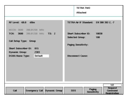
6 Set up the call parameters as explained in "Setting up the call parameters" on page 16. In particular, enter the call setup type (Individual Duplex or Individual Simplex); the Short Subscriber ID and the dynamic group number are not required in an individual, outgoing call.
