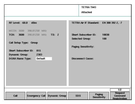
6 Set up the call parameters as explained in "Setting up the call parameters" on page 16. In particular, enter the call setup type; the Short Subscriber ID and the group number are not required in an incoming emergency call.
